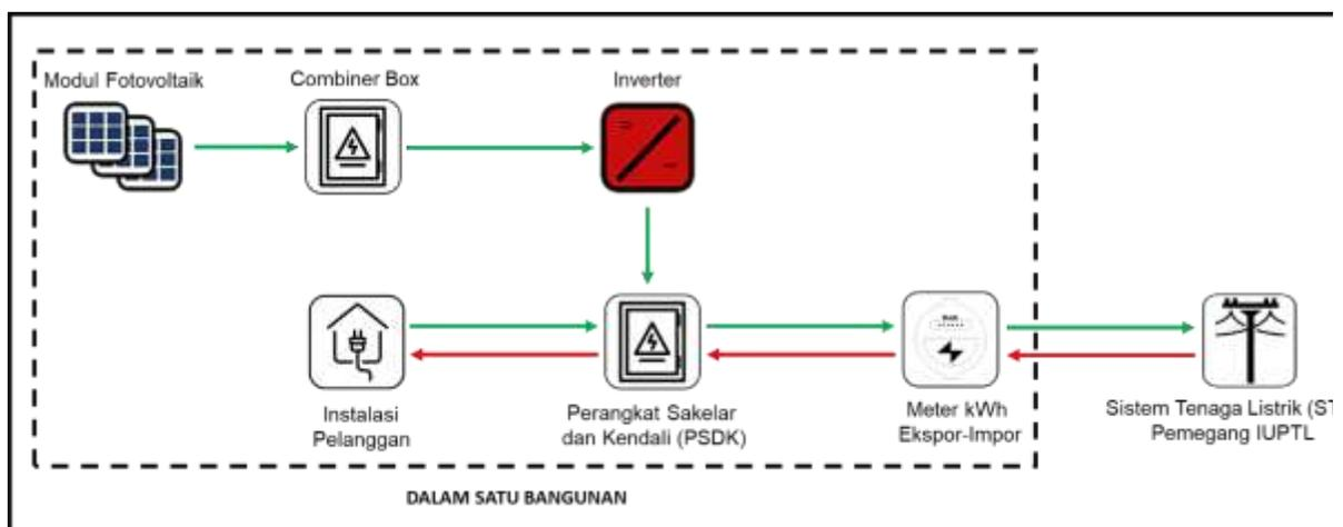
DIAGRAM INSTALASI SISTEM PLTS ATAP DENGAN BATERAI
